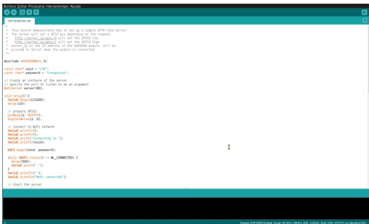
The screenshot shows the Arduino IDE interface with a sketch titled "WiFiAndServer". The code demonstrates how to set up a simple HTTP-like server on an ESP8266 module. It includes setup for WiFi connection, digital pin control, and a basic web server loop. The IDE status bar at the bottom indicates the board is an "Element 8266 Module" and the serial port is "Serial (0) 115200 8N1".
