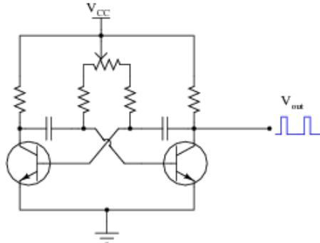
A student desires to use this circuit as the basis for a *pulse-width modulation* (PWM) power controller, to vary the amount of power delivered to a DC load. Since the oscillator circuit is built to produce weak signals and not deliver power directly to a load, the student adds a power MOSFET to switch heavy load currents:
